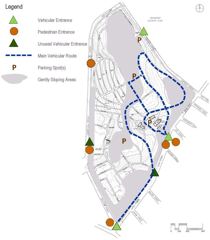
Figure 4.2. Entrances, circulation, parking and accessible slopes.
