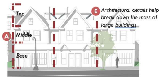
Figure 3: Facade Design Diagram (1 of 4)
