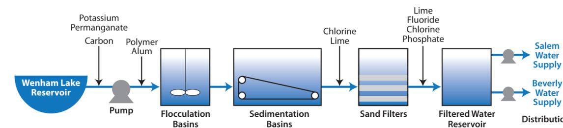
Water from the Ipswich River and the three reservoirs goes to a water filtration plant, operated 24 hours a day, 7 days a week by the Board. The plant removes naturally occurring impurities, as required by federal regulations and good public health practices, and delivers the water to pumping stations owned by the cities of Salem and Beverly. These pumping stations deliver water to your home in pipes owned and maintained by each city water department.
