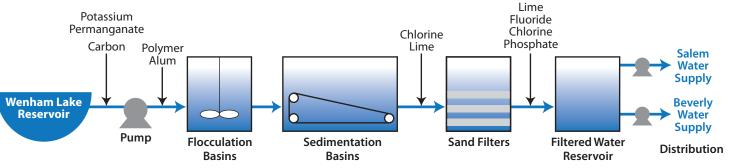
Water from the Ipswich River and the three reservoirs goes to a water filtration plant, operated 24 hours a day, 7 days a week by the Board. The plant removes naturally occurring impurities, as required by federal regulations and good public health practices, and delivers the water to pumping stations owned by the cities of Salem and Beverly. These pumping stations deliver water to your home in pipes owned and maintained by each city water department
