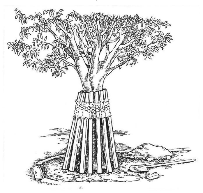
Thick wooden planks tapered to protect trunk and buttress roots at construction sites.
